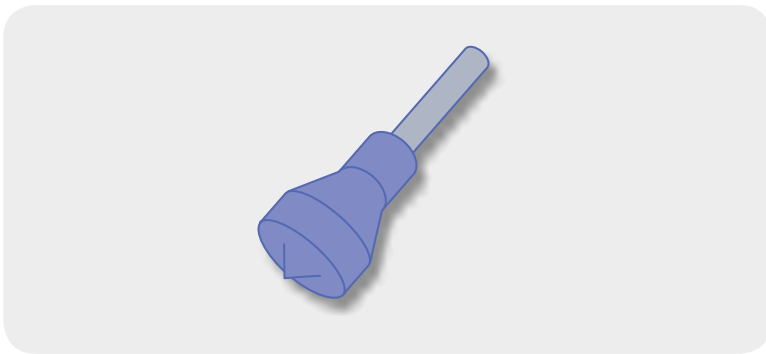
Figure 11: Image of probe-tip illustrating a nipple-tip extrusion
